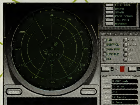
Electronic intercept information is displayed on the SLQ-32 console.
